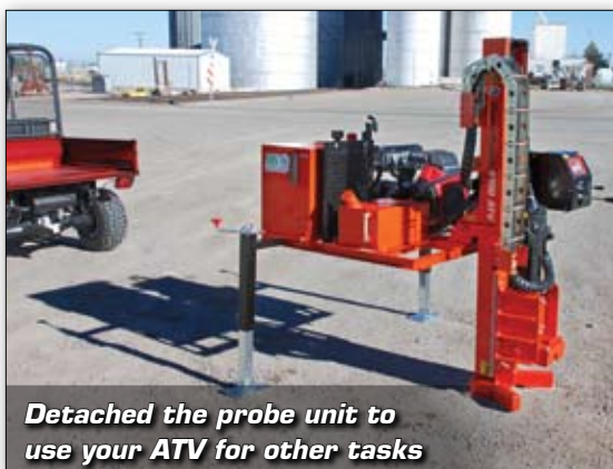
Quick-mount sliderail system for easy storage
